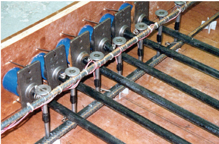
Fig. 2.749: Stud rails can also be used to resist bursting stresses in anchorage zones. The shown headed studs have been instrumented with strain gages to verify their ability to prevent control horizontal splitting at anchorage zones. (Image courtesy of Concrete International, Headed Studs in Anchor Zones of Post-Tensioned Slabs , April 2005.)
